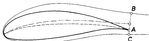
Fig. 1 Equivalent airfoil contour, generated by adding the boundary-layer thickness to the original shape.
